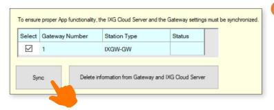
If the sync fails, or the status LED never turns green, confirm both the programming PC and the Gateway have an internet connection. Also, confirm the Default Gateway and DNS settings configured under **Network Settings** are set correctly.
